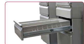
full depth box and file drawers 28" deep [deepest in the industry] 20 gauge 1-piece jacket 18 gauge bottom and uprights & welding of uprights to create rigid box structure heavy forming of drawer sides adds to strength and durability
